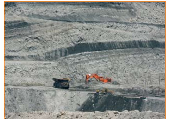
Coal seams are at angles ranging from 17 to 23 degrees, making for difficult extraction.
